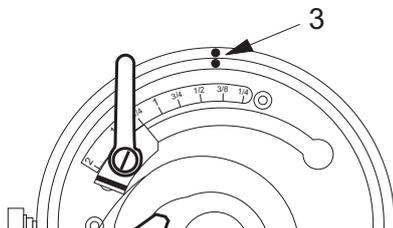
10. Turn the pipe cutter back into its home position.
