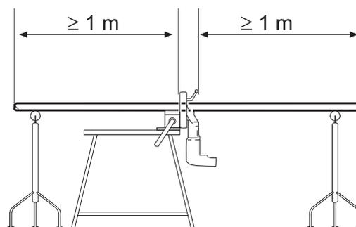
**Important** Use a pipe support for pipes that are over 1 m long.
