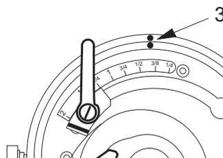
10. Turn the pipe cutter back into its home position.
