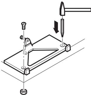
1. Mark and punch the bolt holes on the work bench. Use the quick-mounting base plate as a template.
