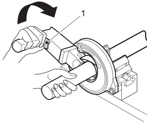
9. Continue to turn rapidly until the pipe has been cut off and the marks (3) on the slide housing and vise housing are aligned.
