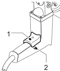
8. Carefully turn the pipe cutter clock-wise until the wall of the pipe has been pierced through.
